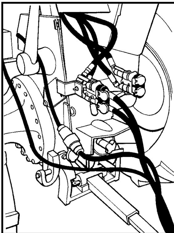
Pik Rite designs the harvester for operation in the *closed center flow mode*.
