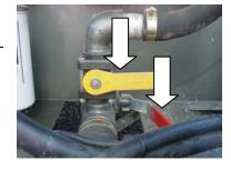
Do not let slurry in the application system for prolonged periods i.e., overnight. The mulch will continue to absorb water and expand, causing the system to plug.
