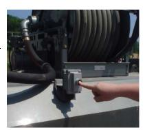
The hose reel is a 12vdc rewind system that allows the operator to adjust spring tension to create more or less drag on the reel. The reel does not have a locking feature so it is important that the nozzle be securely tucked into the bottom of the reel when transporting. Proper tension adjustment will not allow the reel to unravel during transport.
