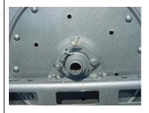
A 70 amp breaker protects the hose reel motor from overload and can be reset by pressing the red button as shown.
