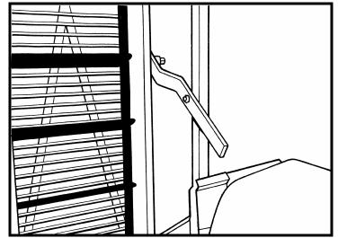
5. Remove discharge conveyor main cylinder from the transport position. Install in working position. Remove the transport bar & store for your next use. Raise & lower the discharge conveyor slowly, watching for any binding or misalignment. See *Illustration D.*
