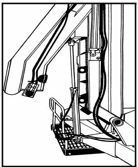
6. Install the basket shields. Be sure the basket shields do not catch on the conveyor frame when moving the conveyor up & down; check to be sure that the conveyor belt will run smooth. See Illustrations E and F.
