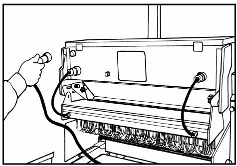
Before connecting power plug at electronic box, check polarity at plug on electronic sorter (<u>if polarity is wrong</u>, it may burn out the box):
