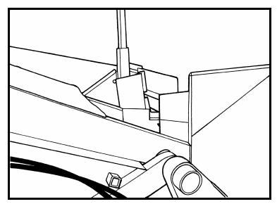
8. Pull out the decking & secure with the catches.
