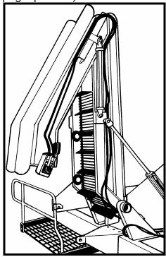
Install the transport bar to canopy post & discharge conveyor. This will hold discharge conveyor in upright position until main cylinder can be repositioned. See *Illustration C.*
