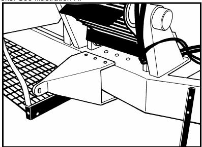
3. Remove the  $\frac{1}{2}$ " bolt securing the transport bar to the sorting table post. Remove the transport bar from the discharge conveyor. *See Illustration B.*
