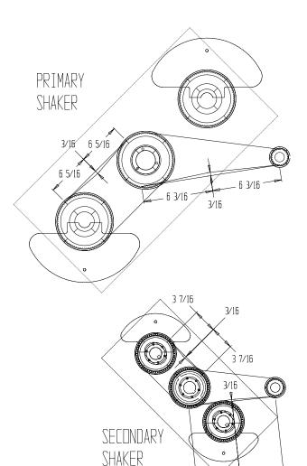
When belt replacement is necessary, refer to the Pik Rite service video for belt installation and weight timing procedures. Note that pulleys must be parallel. Misalignment causes uneven pressure on the teeth of the belt, uneven loading of the tensile member and extreme edge wear on the belt which can result in premature belt failure. Never pry or otherwise force belts onto pulleys as this can result in permanent damage to the belt.
