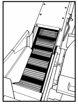
**CAUTION:** The basket shield and rear tomato saver shield must be installed after the hand-sort conveyor is folded down.
