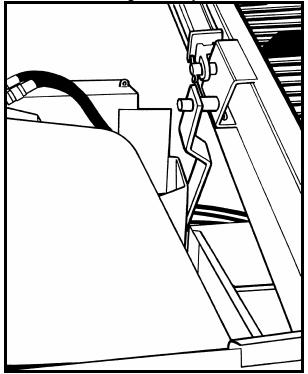
4. Extend the discharge conveyor main cylinder (this will lift the discharge conveyor
