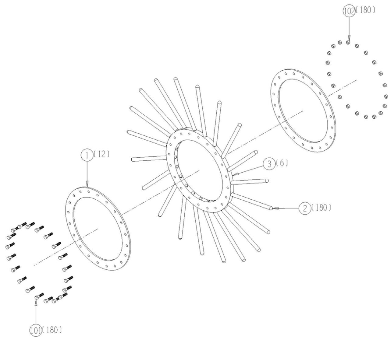
1009-05-18 Shaker Spacer Tube (per shaker) Assembly
