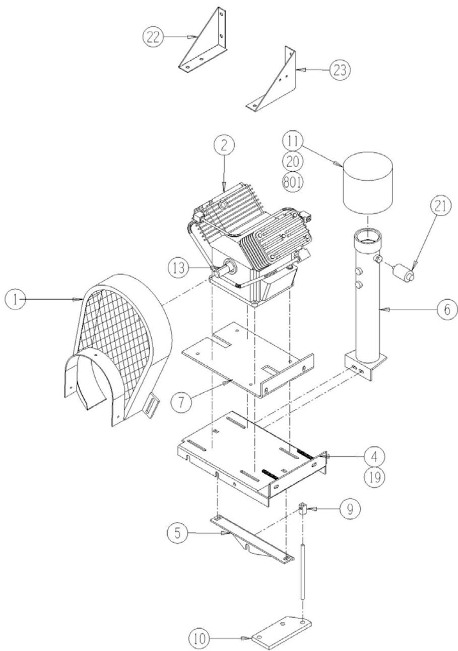
**1009-12-02 Air Tank Assembly & Pneumatics**
