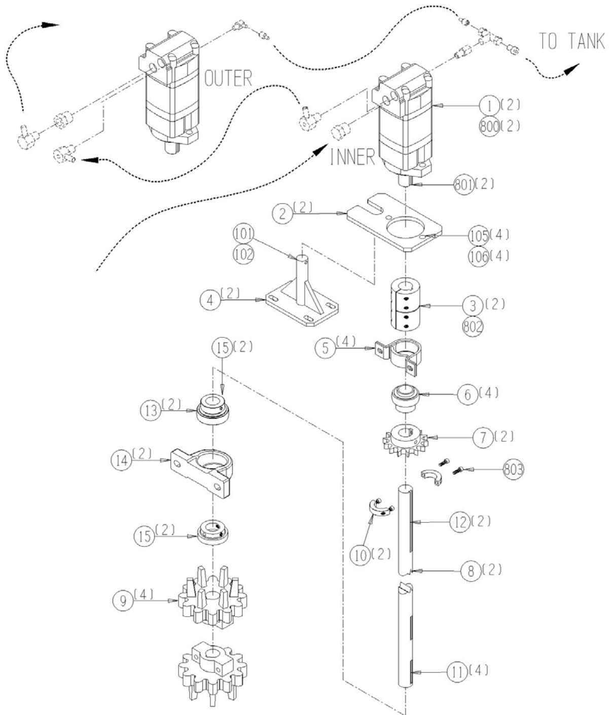
1009-02-03      Disk Header 34" Disk Shaft Assembly
