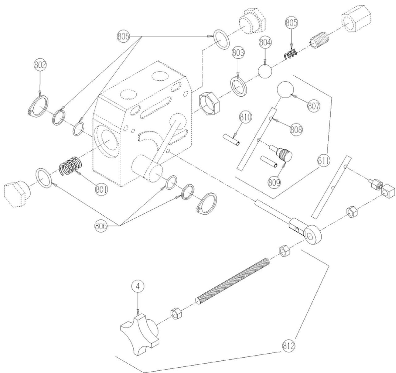
1009-80-05      Hydraulics, Relief Valve Parts Assembly
