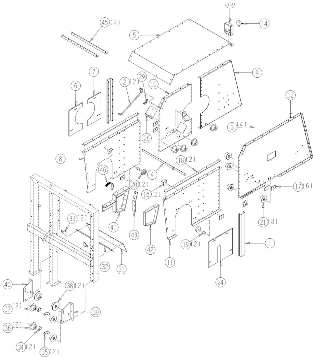
1009-04-51 Optional Shaker Chamber Box Shield Assembly
