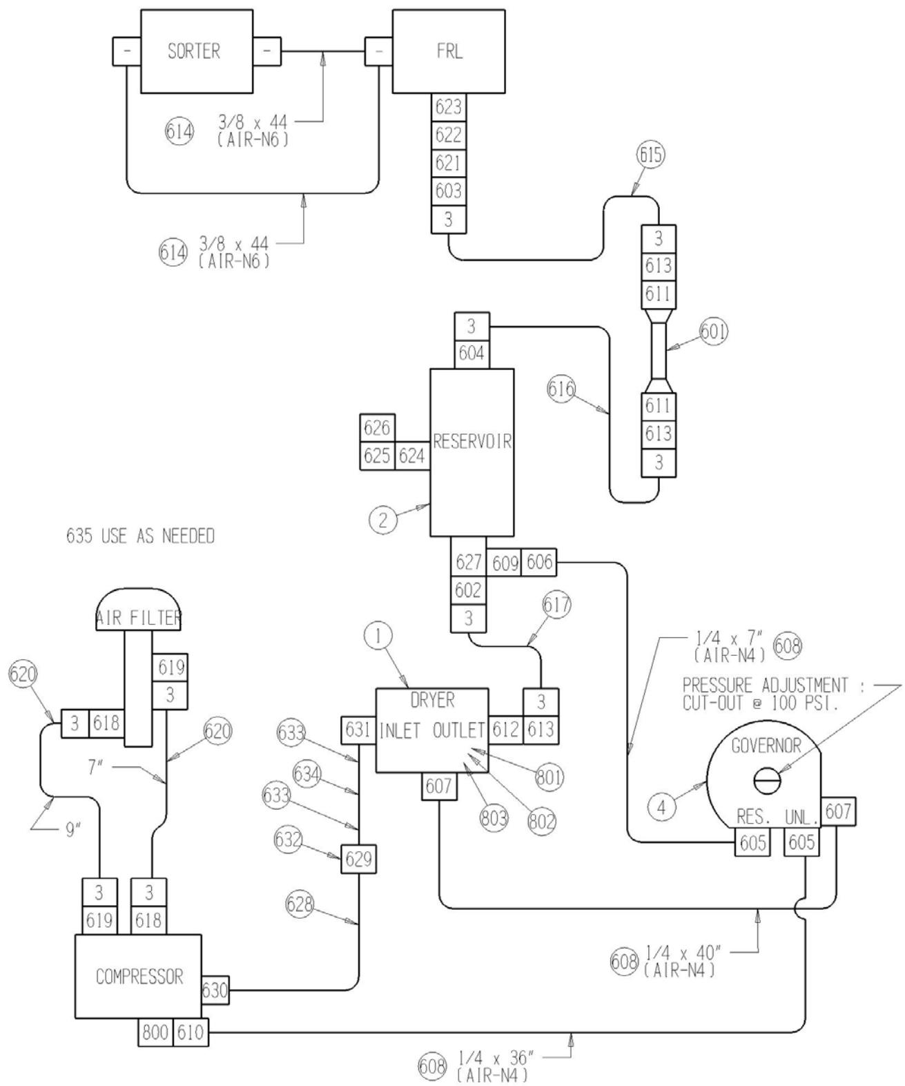
**1009-12-03 Double Pump Air Compressor Assembly**
