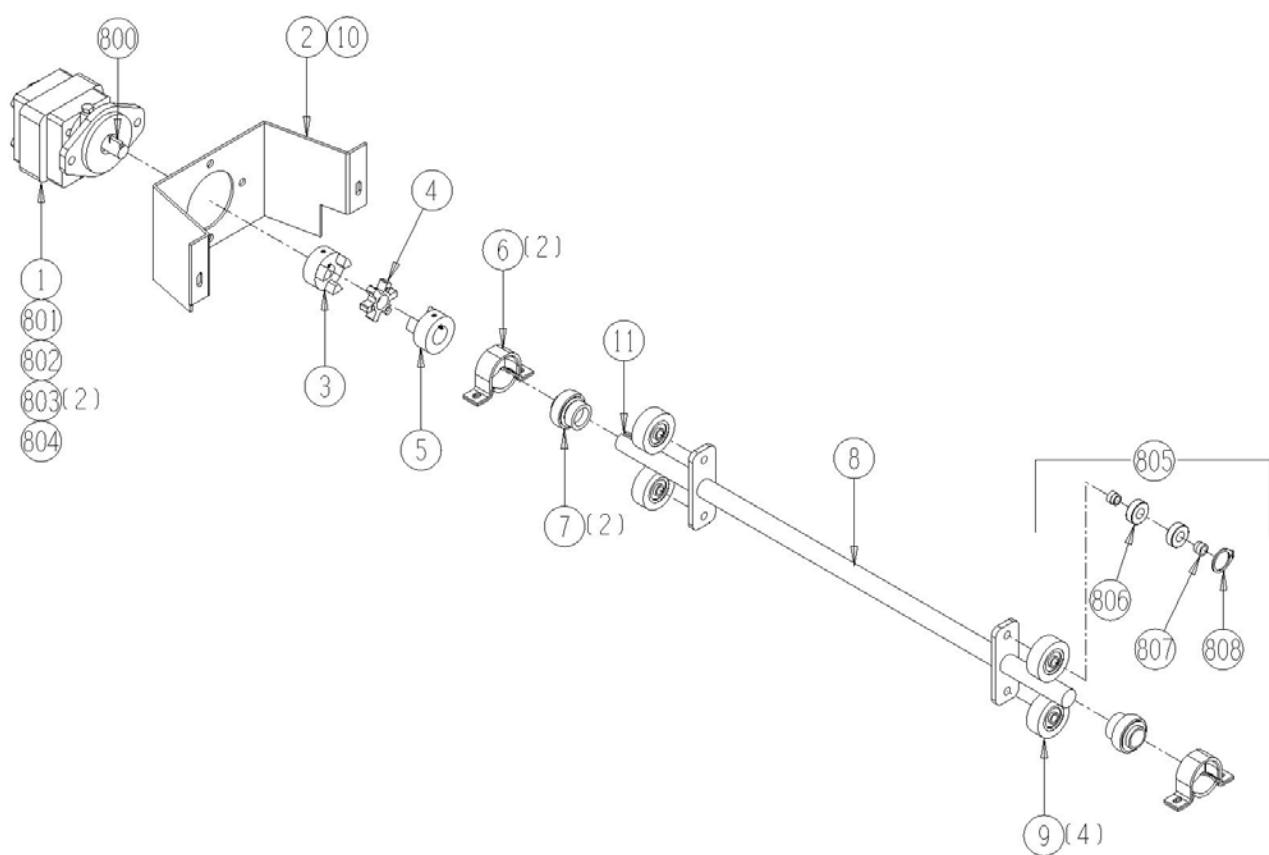
1009-03-12 Secondary Header Frame Assembly Less Vine Assist
