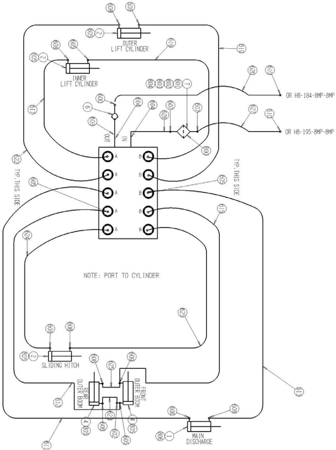
1009-14-03H      Hydraulic Control Valve, No Leveling
