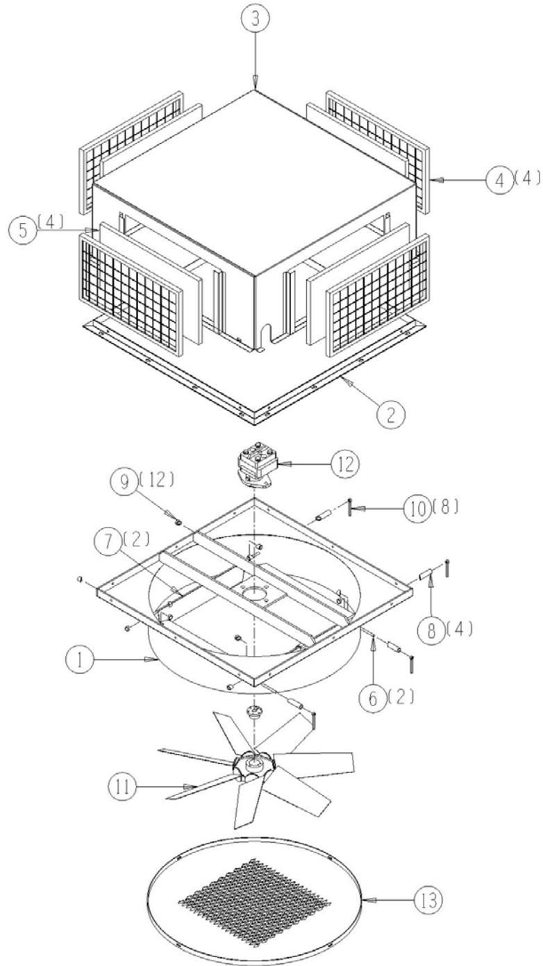
1009-11-03H Enclosure Fresh Air Fan Hydraulic Assembly
