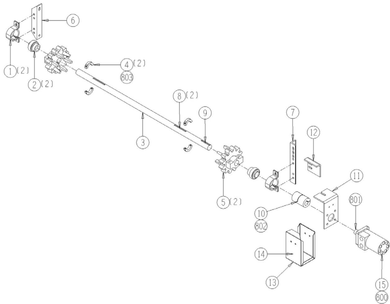
1009-08-07 Opt. Elevation Conveyor Bar Cleaner Assembly
