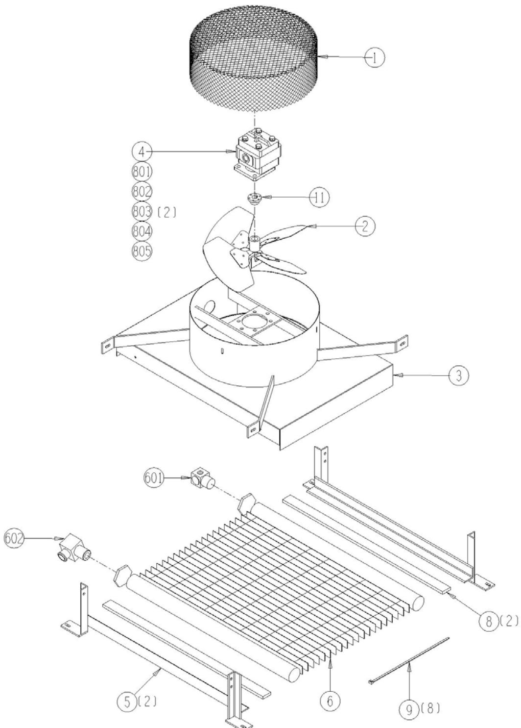
1009-13-04 Double Pump Oil Cooler Assembly
