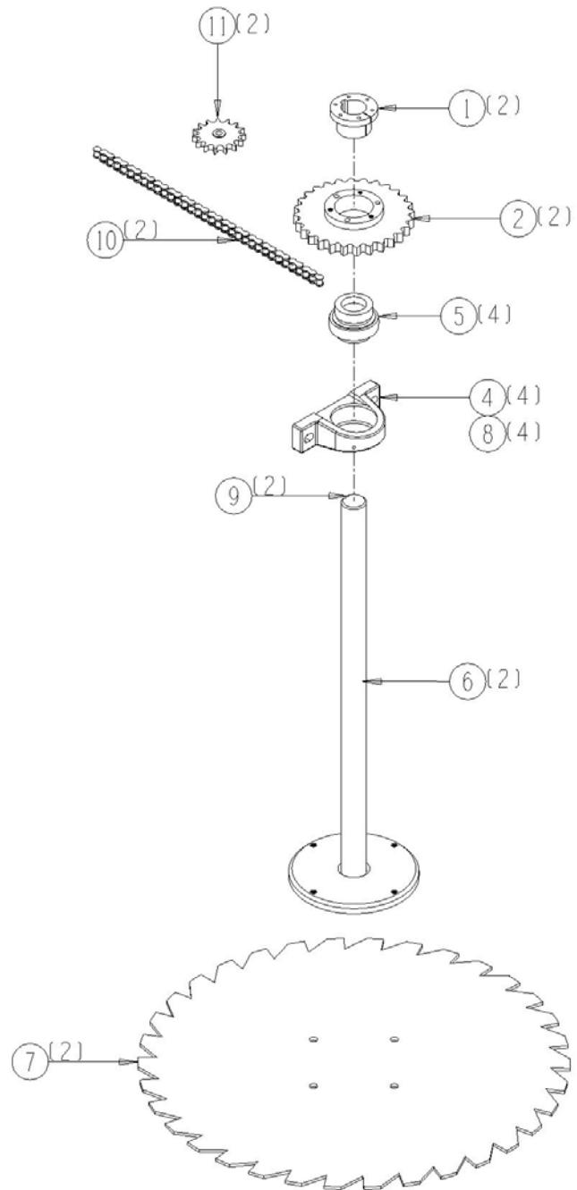
1009-02-04 Disk Header 36" Disk Shaft Assembly
