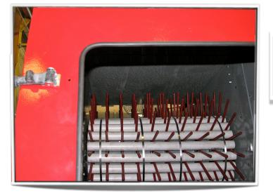
The 240 Harvester features a dual-forced balance shaker system that gently separates the fruit from the plant.
