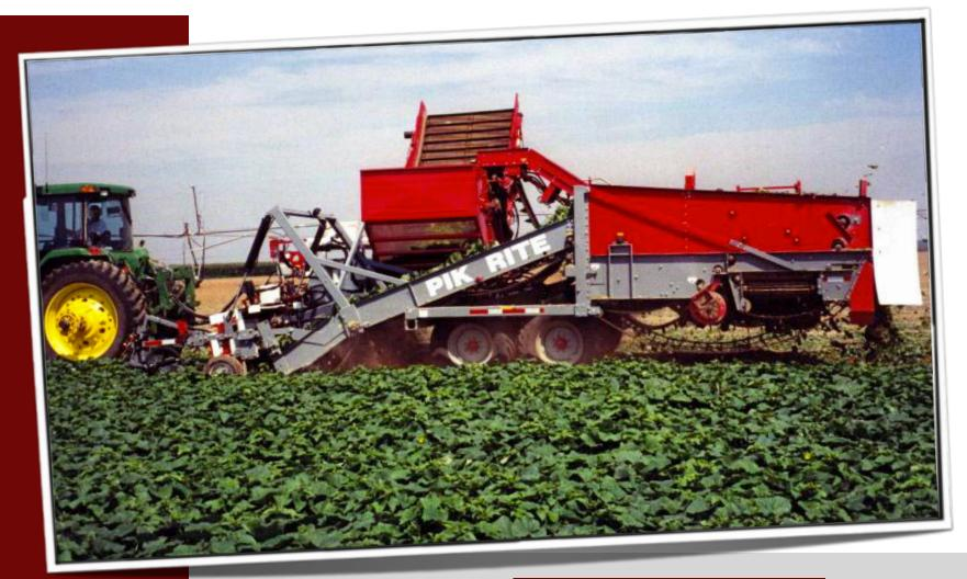
The 3000 Cucumber Harvester runs at 2 to 3 MPH and features incredible advantages not found in competitors' models, including a large (125 bushel) live-bottom bin for speedy on-the-go unloading.
