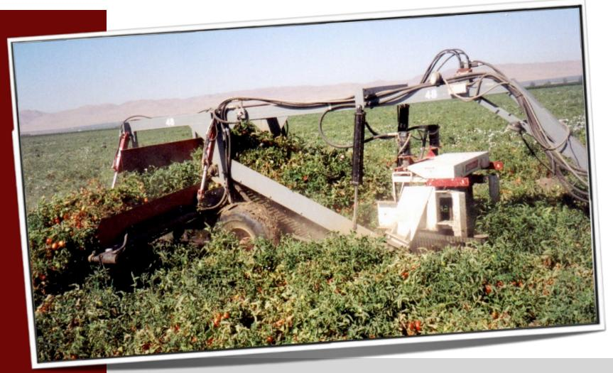
The 6000 Vine Diverter allows you to relocate fruit and vines from one row to an adjoining row to assist in opening a field for harvest or to reduce the number of trips required by the harvester.
