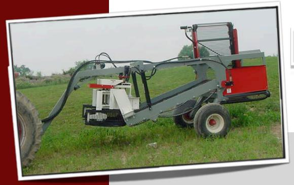
The Pik Rite 6000 Vine Diverter can be run at speeds of approximately 3 to 6 miles per hour.
