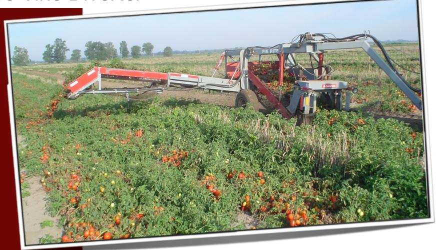
Pik Rite's 6200 Vine Diverter allows you to relocate fruit and vines from one row to an adjoining row to assist in opening a field for harvest or to reduce the number of trips required by the harvester.
