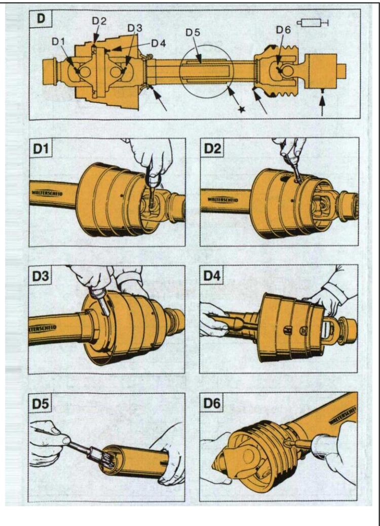
**NOTE:** Lubrication step D5 is only necessary when driveline does not have grease fitting. Separate front and rear halves of driveline and brush with grease.
