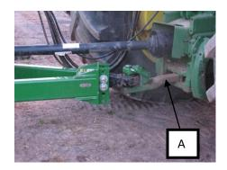
A tractor drawbar support is required on tractors with a drawbar size of 1-1/2 x 3 in. minimum
