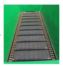
Remove material buildup from endgate panel. Keep endgate arms clean to prevent freezing to side rails.
