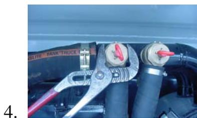
Once the desired, regulated, pressure has been attained, simply secure the outer lock nut that was loosened in step #2.
