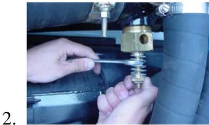
Holding the inner hex nut, closest to the main housing, turn the knurled nut clockwise for more vacuum in the tank and counterclockwise for less.
