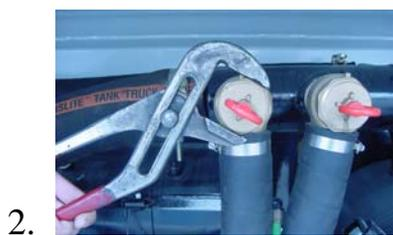
Using a wrench, loosen the large, outer nut to allow for adjustment.
