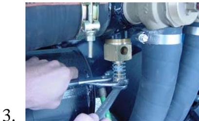
Once the desired vacuum has been attained, simply hold the knurled nut firmly with pliers while tightening the outer hex nut securely against it.
