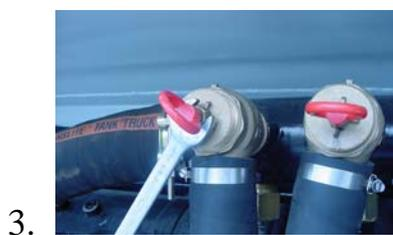
With a 5/8" wrench, turn the small hex nut clockwise for more pressure in the tank or counterclockwise to relieve pressure for less pressure in the tank. Never adjust this valve when pressure is in the tank, the end could fly off causing injury or death.
