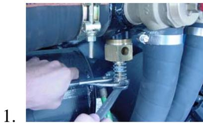
While securing the knurled nut, loosen the hex nut at the end of the spring.
