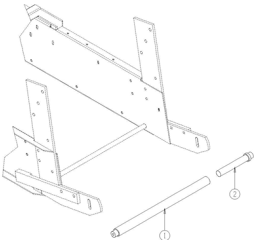
12011-03-11 Header Conveyor Vibrator Shaft Assembly
