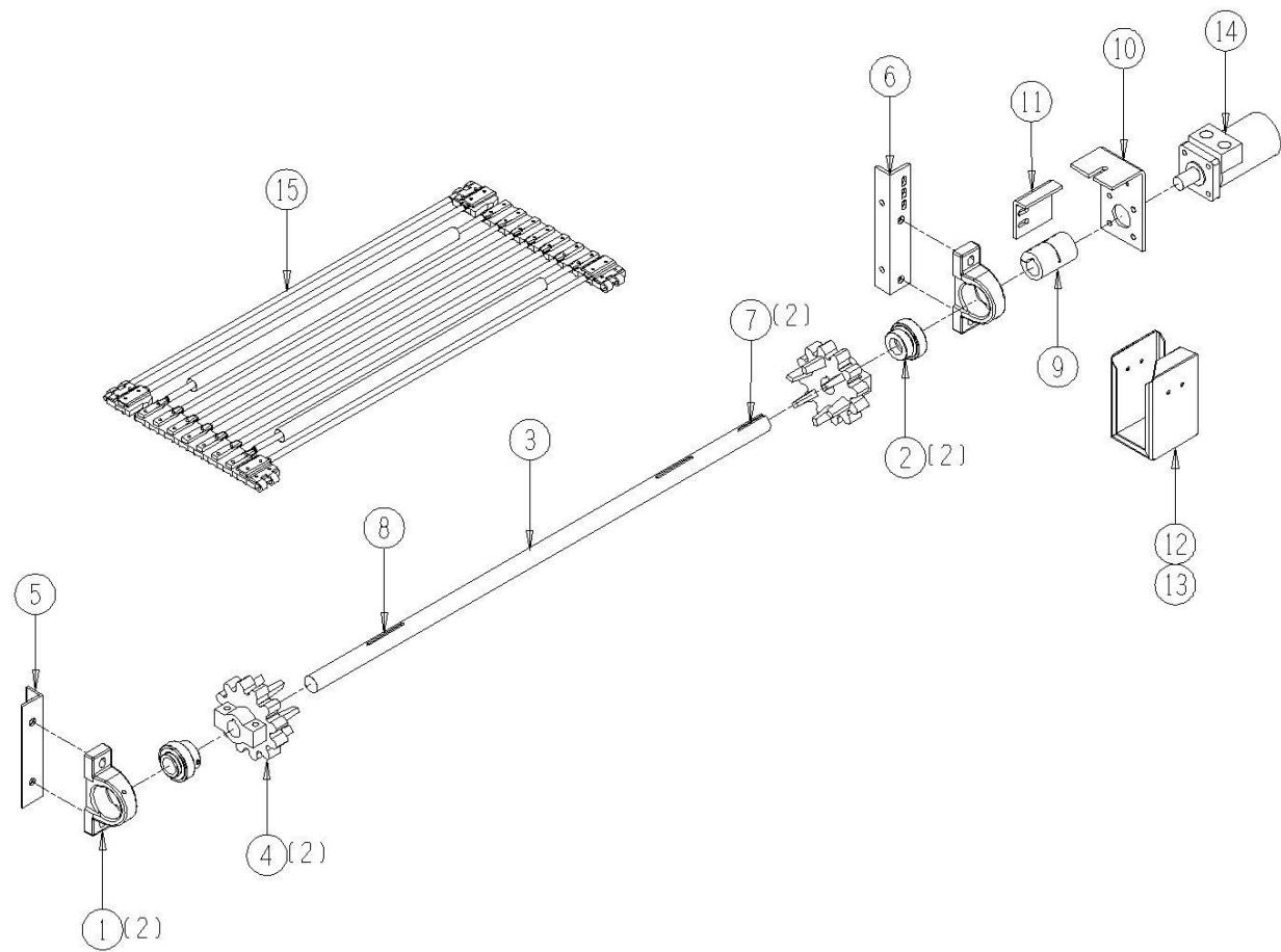
12012-08-07 Opt. Elevation Conveyor Bar Cleaner Assembly
