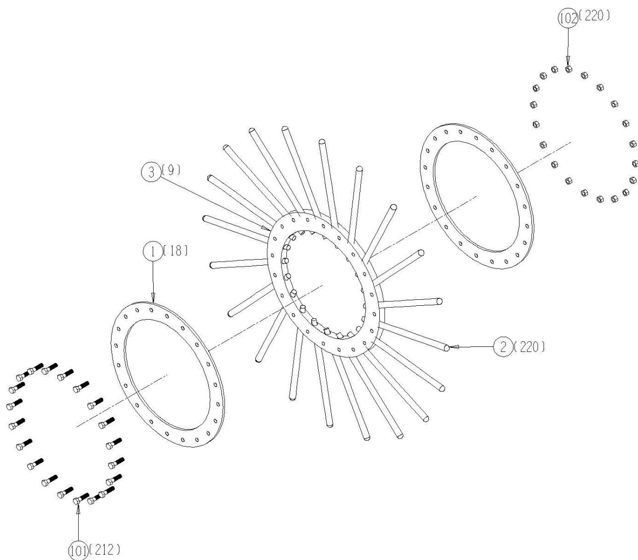
12011-04-06 Shaker Spacer Tube Assembly
