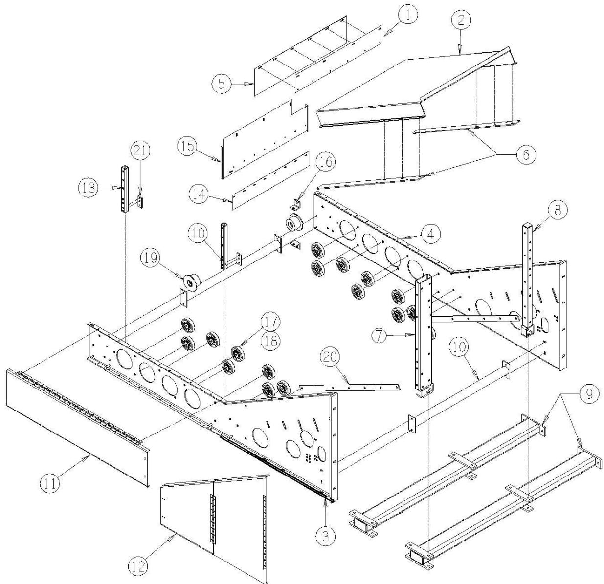
12012-08-03 Elevation Drive Shaft Assembly
