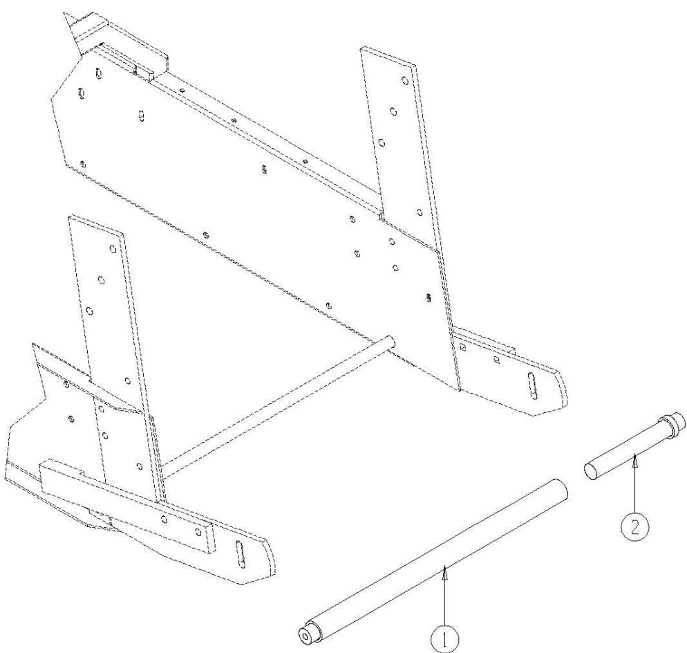
12011-03-11 Header Conveyor Vibrator Shaft Assembly
