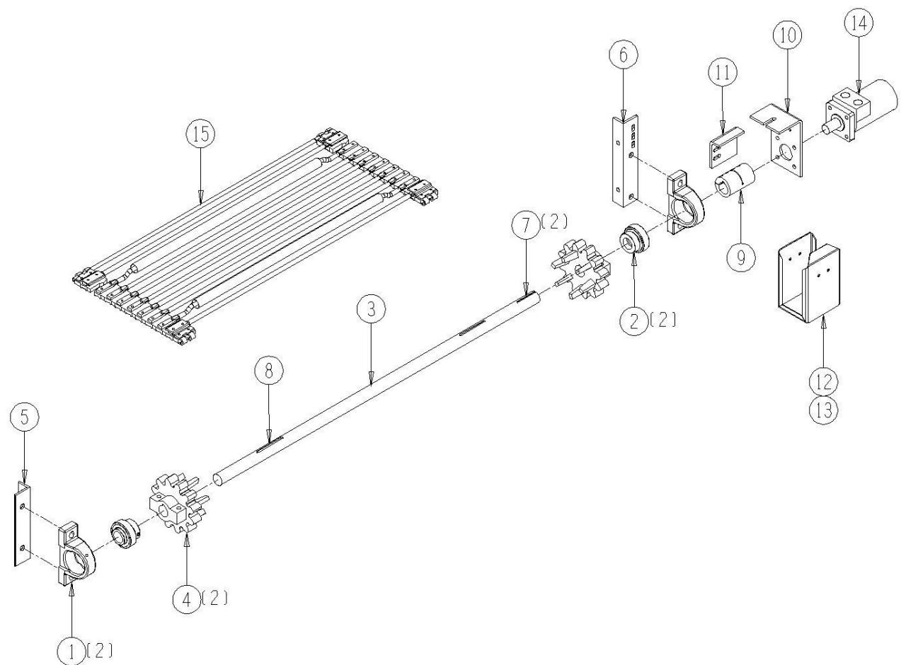
12011-08-07 Opt. Elevation Conveyor Bar Cleaner Assembly
