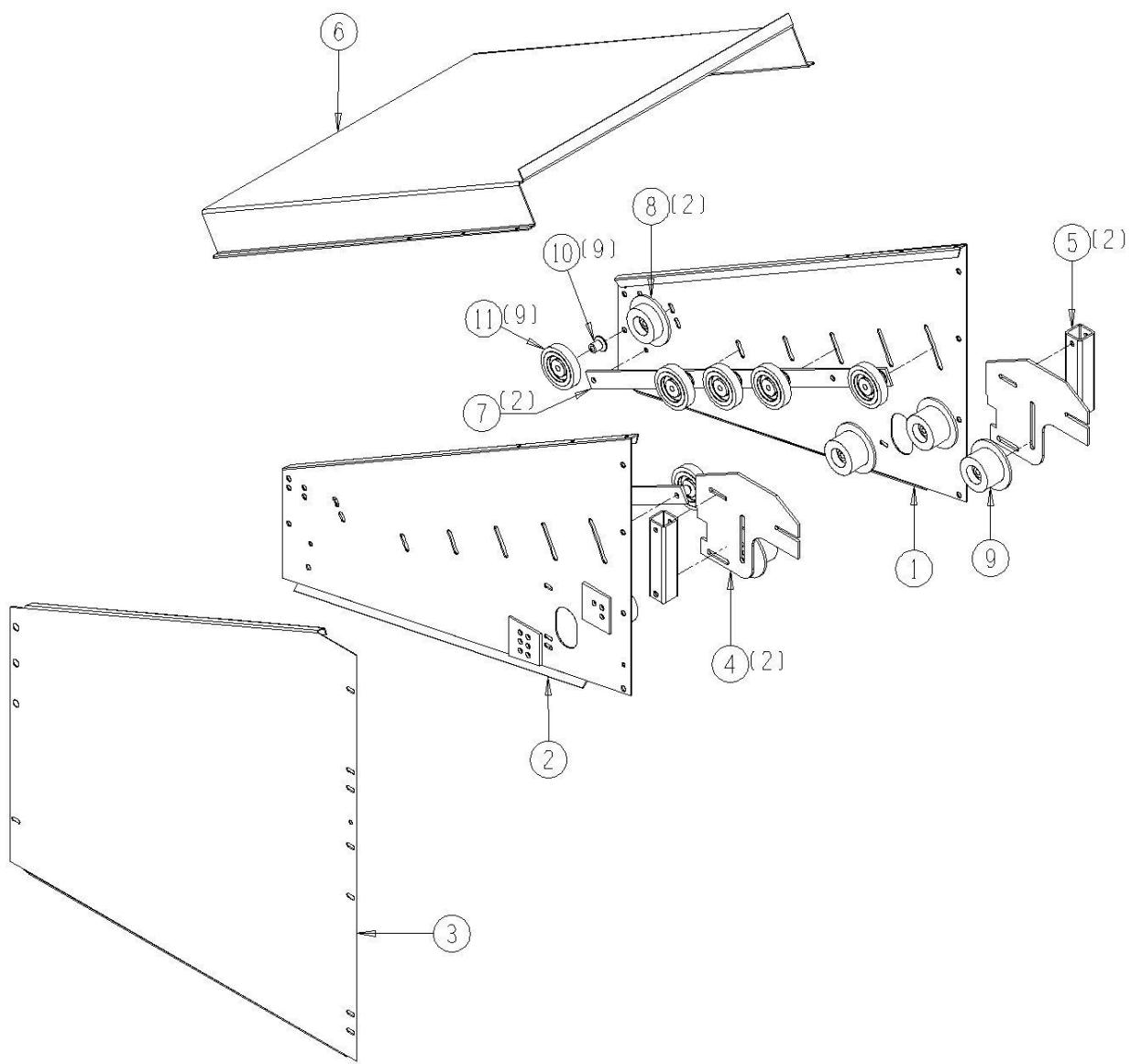
12011-08-03 Elevation Drive Shaft Assembly
