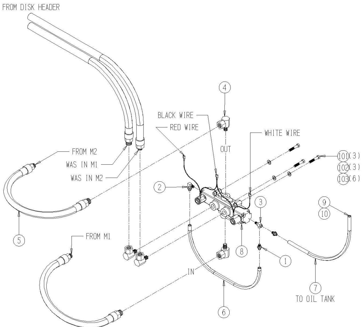
11010-15-21      Electronic Flow Control (3/4" Lines) Assembly
