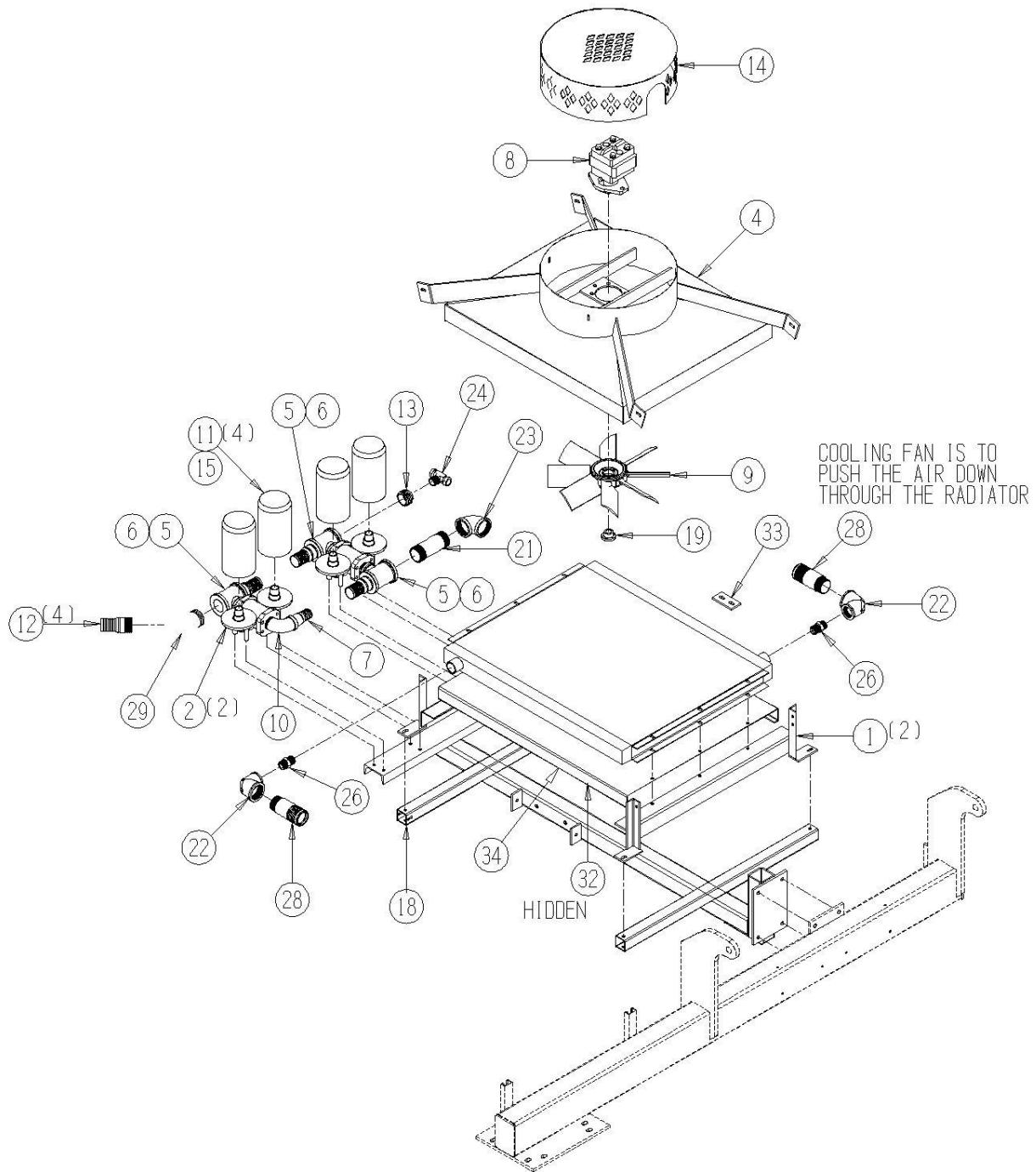
11010-15-04 Shaker Rot. Valve Sect. Assembly w/Fresh Air Fan
