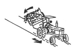
Braking to stop towed loads from transport speeds can cause the towed load to swerve and upset. Reduce speed if towed load weighs more than the tractor and is not equipped with brakes.
