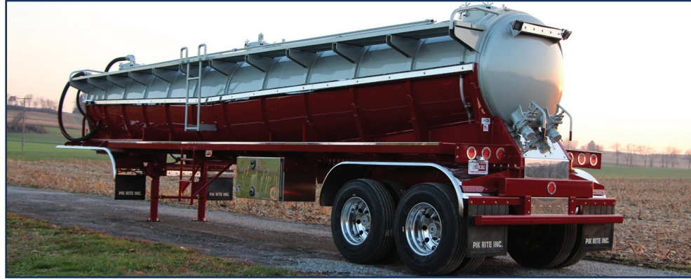
PAINTED ALUMINUM 7,000-GALLON DOUBLE CONICAL VACUUM TANK TRAILER
