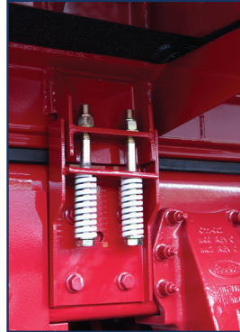
OVERLAPING MOUNT BRACKETS SECURED BY 4 BOLTS FOR EXTRA SAFETY
