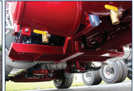
ROBUST PUMP STAND IS MOUNTED TO BOTH FRAME RAILS
