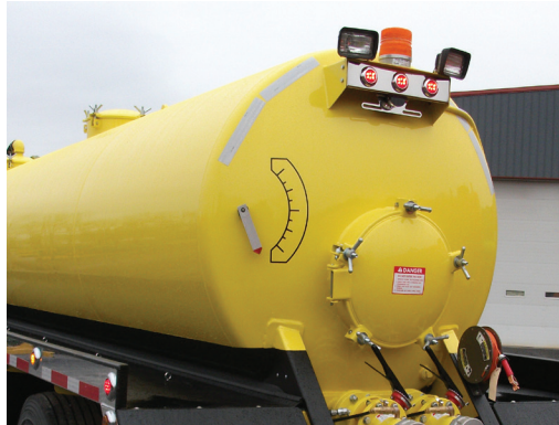
FLOAT BALL LEVEL INDICATOR
