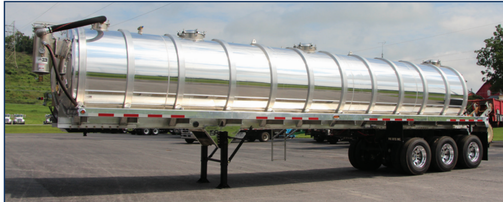
HIGH CAPACITY 9,000-GALLON ALUMINUM TRI-AXLE VACUUM TANK TRAILER
