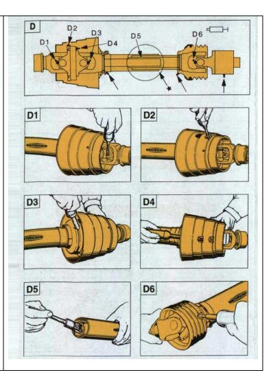
**<u>NOTE:</u>** Lubrication step D5 is only necessary when driveline does not have grease fitting. Separate front and rear halves of driveline and brush with grease.
