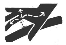
Avoid the hazard by relieving pressure before disconnecting hydraulic or other lines. Tighten all connections before applying pressure.
