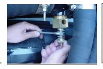
Holding the inner hex nut closest to the main housing, turn the knurled nut clockwise for more vacuum in the tank and counterclockwise for less.
