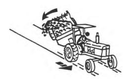
Braking to stop towed loads from transport speeds can cause the towed load to swerve and upset. Reduce speed if towed load weighs more than the tractor and is not equipped with brakes.
