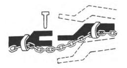
Using the appropriate adapter parts, attach the chain to the tractor drawbar support or other specified anchor location. Provide only enough slack in the chain to permit turning.
