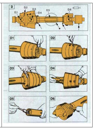
NOTE: Lubrication step D5 is only necessary when driveline does not have grease fitting. Separate front and rear halves of driveline and brush with grease.
