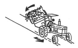
Braking to stop towed loads from transport speeds can cause the towed load to swerve and upset. Reduce speed if towed load weighs more than the tractor and is not equipped with brakes.
