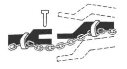
Using the appropriate adapter parts, attach the chain to the tractor drawbar support or other specified anchor location. Provide only enough slack in the chain to permit turning.
